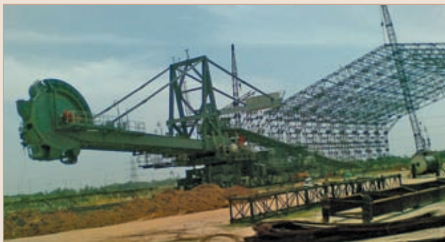
Stacker cum Reclaimer, 3000 TPH stacking and 1500 TPH reclaiming, MECON
