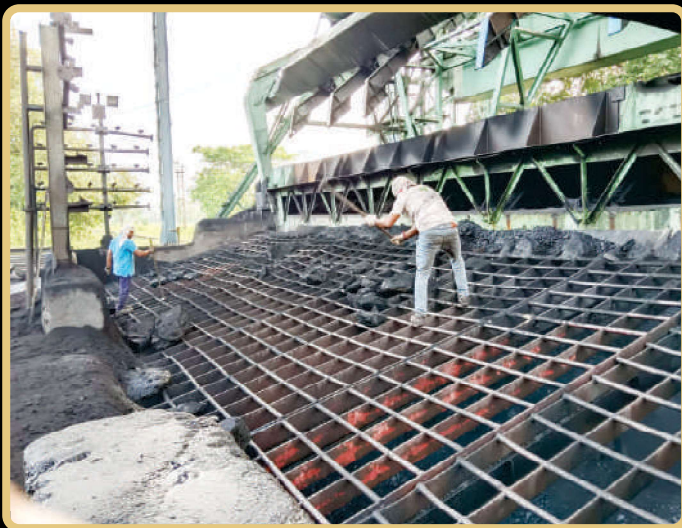
Oversized coal boulders are being manually broken at the plant's hopper following unloading at the tipplers
