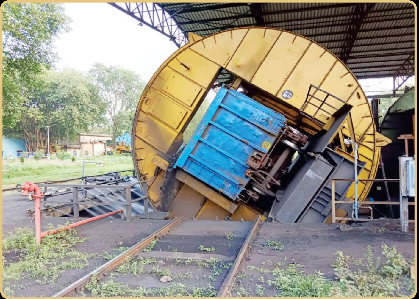
Wagon tippler: Bandel Thermal Power Station, under West Bengal Power Development Corporation is looking to modify the existing wagon tipping arrangements to handle higher number of wagons. The facility has got two old tippler arrangements installed and commissioned in 1962 from Hely & Patterson Co USA, having capacity of 100 tonne, with time taken per cycle of 130 sec, 25 HP (380V/ 40 HP Motor
